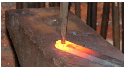
Making the rivet holes
